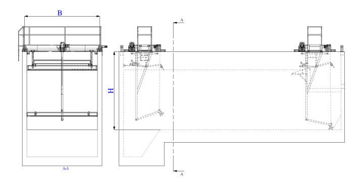
Inclination of the bridge:Power load:Speed of the bridge:Tread (B)L/200, L/4000,37-0,55 kW0,03 m/sto 3-15 m
