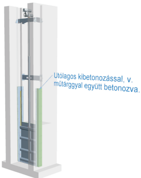
Embedded in concrete
